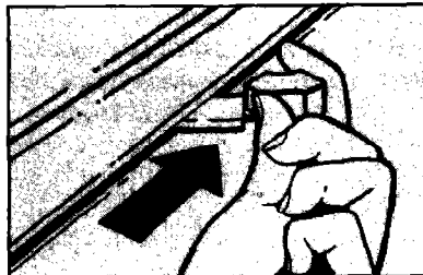
5. Lock the oven door by moving the Lock Lever all the way to the right. When it is all the way over, the Clean Light will come on. If the Clean Light doesn't come on, the lever isn't all the way over and the cleaning cycle won't start.
